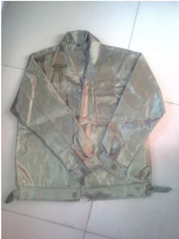
Above: a dome made of basalt fibers Left: a coat made of basalt fibers
