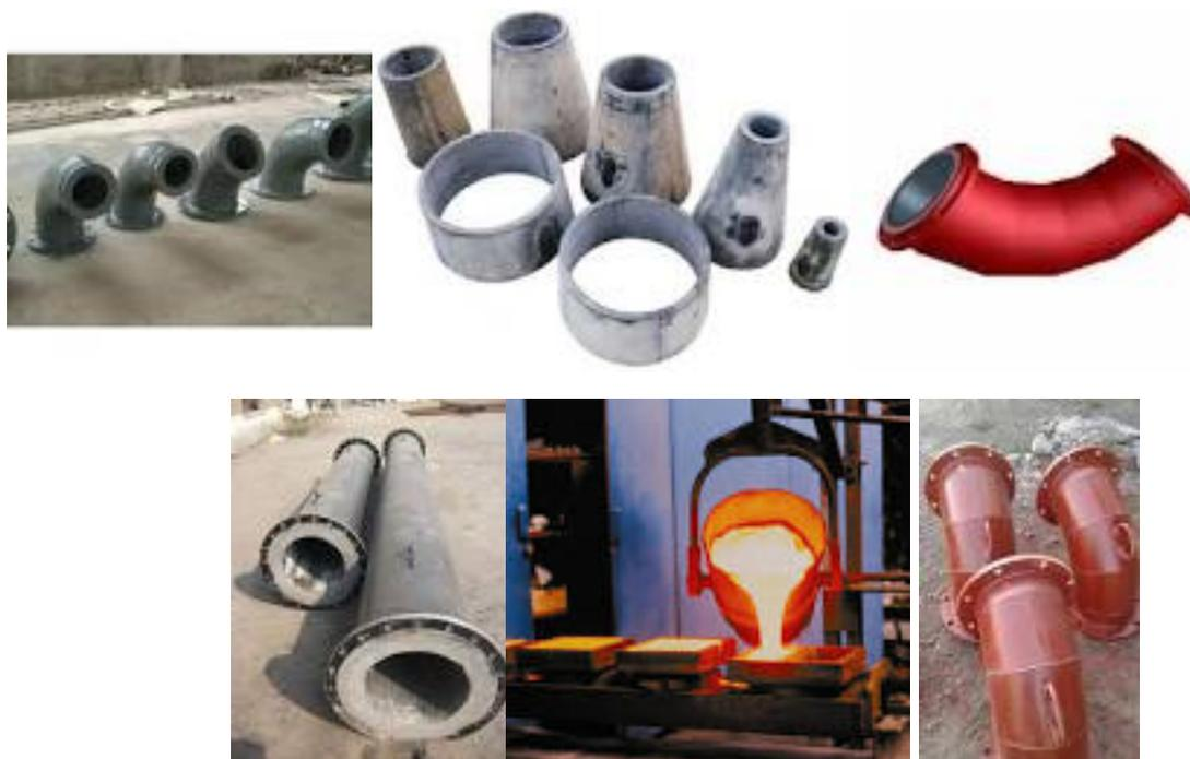
Various forms of abrasion-resistant cast basal pipes, for handling moon dust
