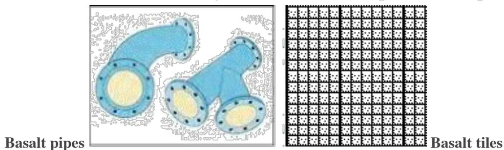
**Number 1, hands down, is that cast basalt pipes, tubes, and chutes - are the only pipes that abrasive moon dust powder will not etch away until they leak.**
